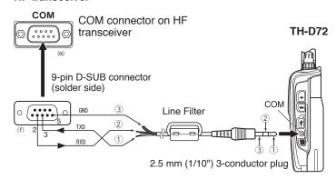
Attach the line filter to the cable.
