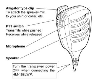
**NEVER** immerse the connector in water. If the connector becomes wet, be sure to dry it BEFORE attaching it to the transceiver.
