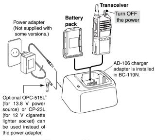
\*CAUTION: NEVER connect the OPC-515L to a power source using reverse polarity. This will ruin the battery charger. White line: (+) Black line: (-)
