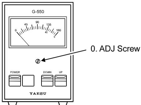
Press the **UP** switch to align the 180° markers on the rotator. The meter should now point precisely to 180° (right edge of scale). If not, adjust the Full Scale ADJ potentiometer on the rear panel so that it does.
