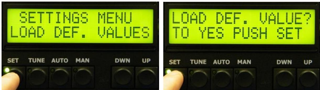
Then select if you want to erase all settings (pressing TUNE) or just one setting value (SET button). In the case of resetting a single parameter use UP / DWN to select which option and confirm by SET.
