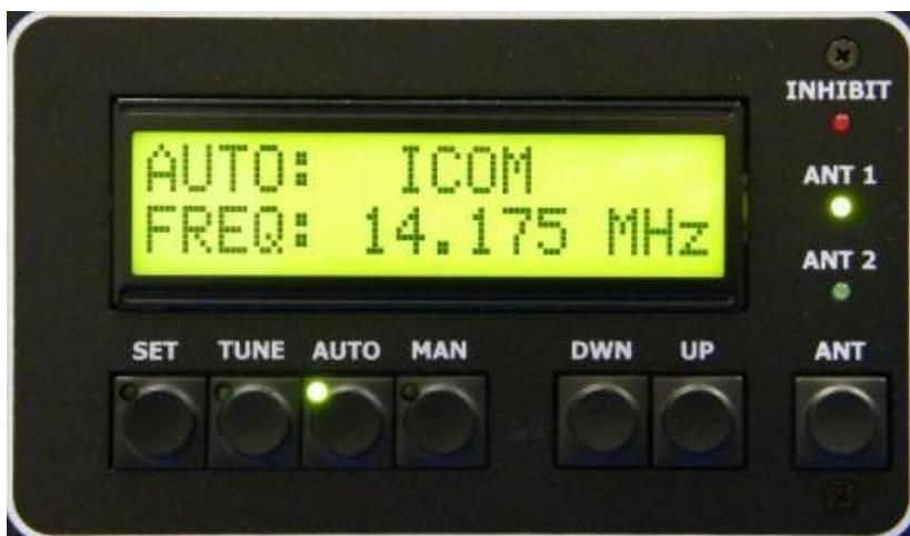
**INHIBIT** Indicates interruption of transmission during the tuning process of the PA. If indicated by RED LED then PA is in STBY mode. If during a retune operations within the same BAND then the PA will retune according to the frequency of
