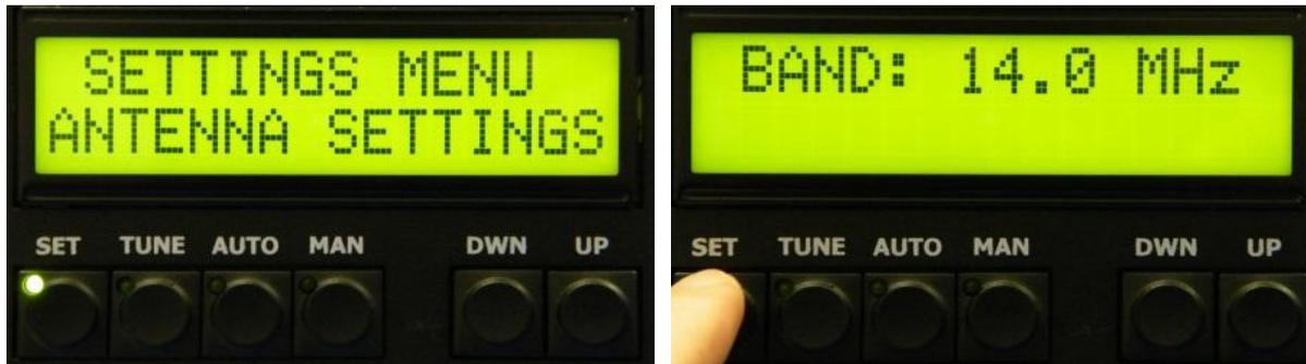
Then select how many antennas you want per current band (1 or 2) and always confirm your selection by pressing SET. The by scrolling UP / DWN you assign which PORT is used on your external antennas switch for this particular antennas. (ANT 1 ON PORT 01).
