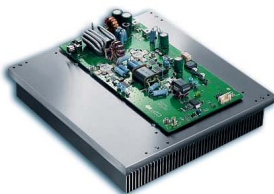
PA unit and large heat sink
